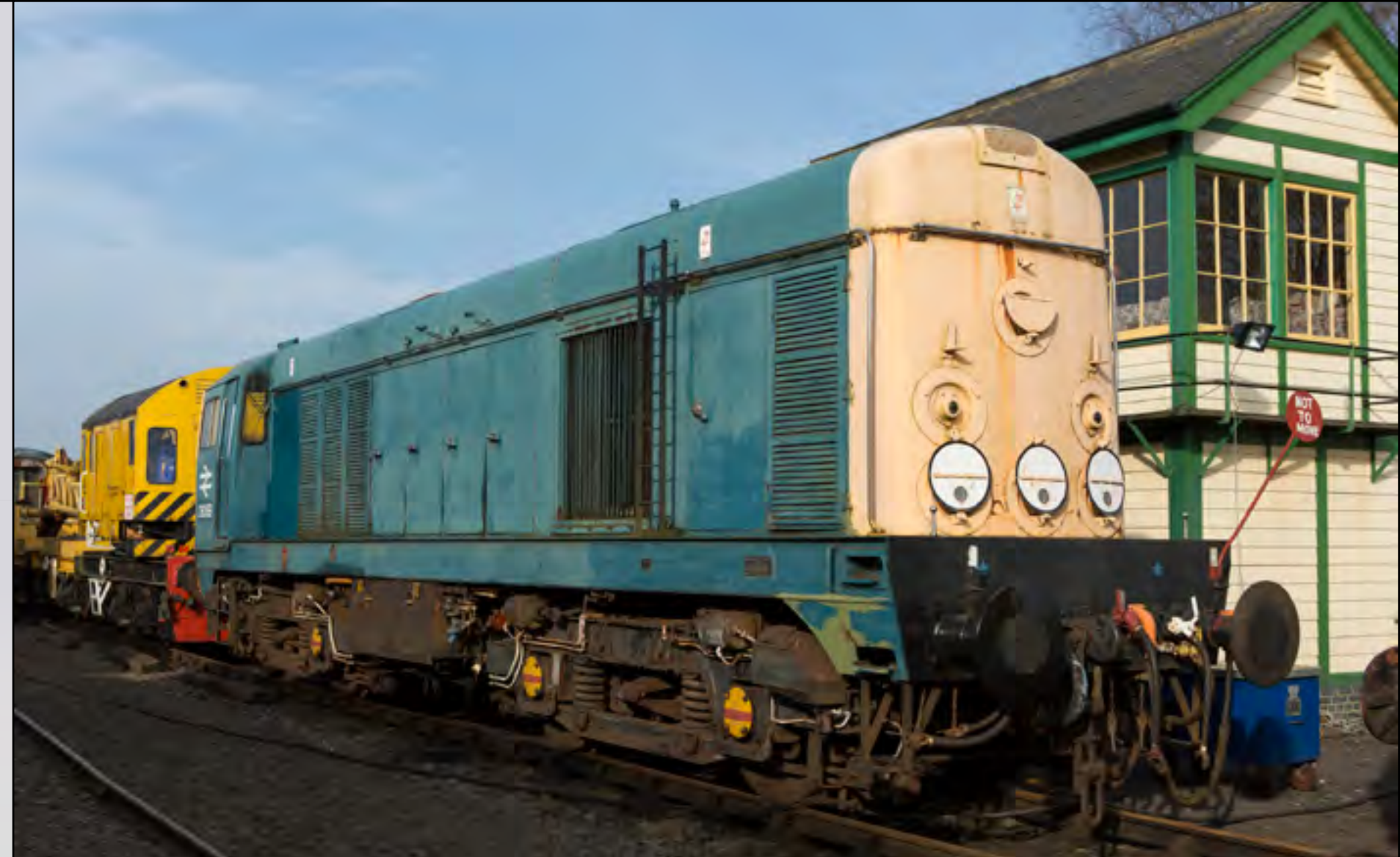
Right: Class 20 No. D8069 is seen next to the Mid Norfolks 10t 4w self-propelled diesel crane, built by Thomas Smith & Sons (Rodley) Ltd, No. DR81330. Jon Jebb
