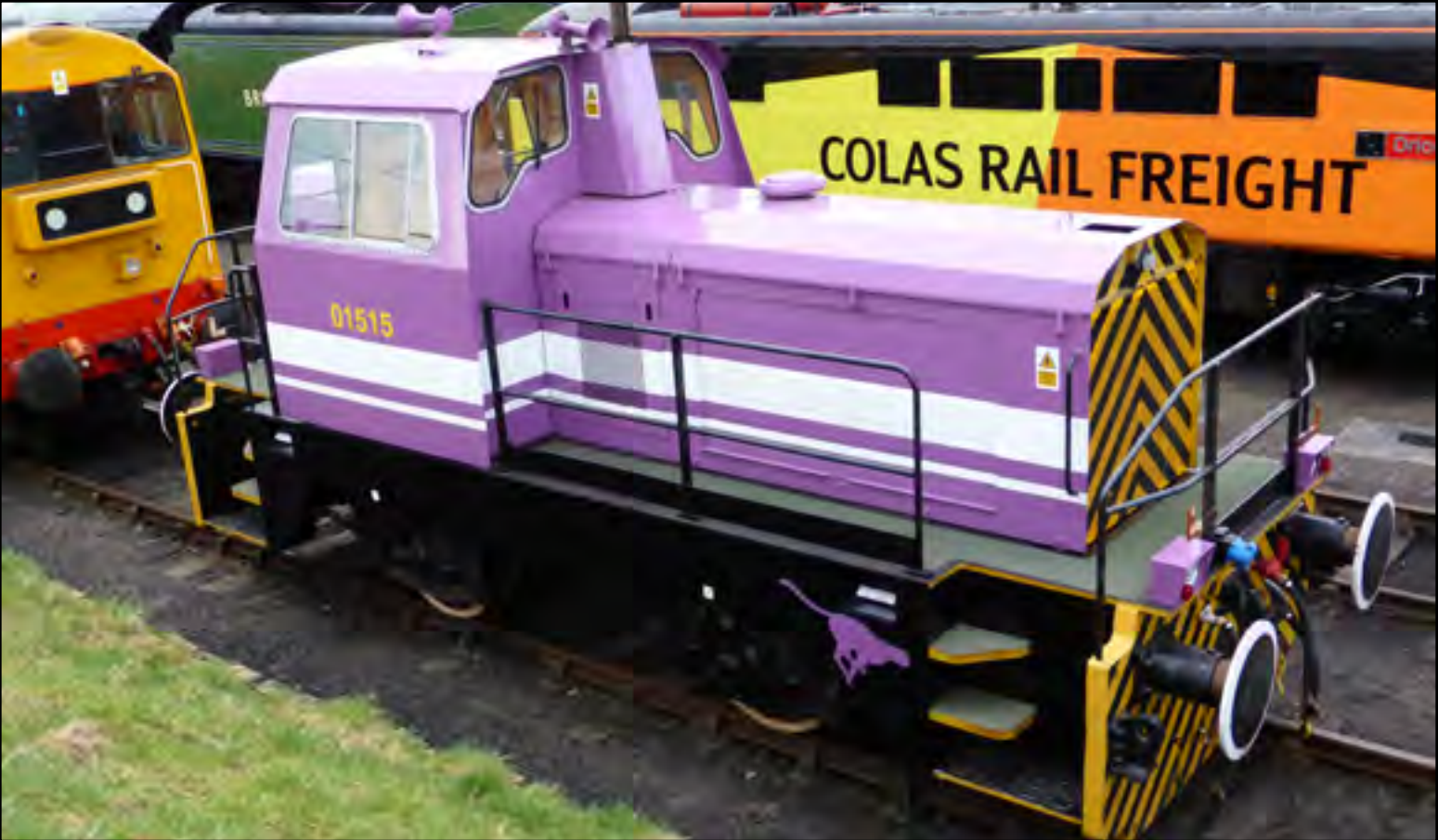
Above: Recently overhauled Thomas Hill 321V 4wDH (1987) No. 01515 shunter, one of the Harry Needle fleet, awaits final attention on March 1st. Andrew Wilson
