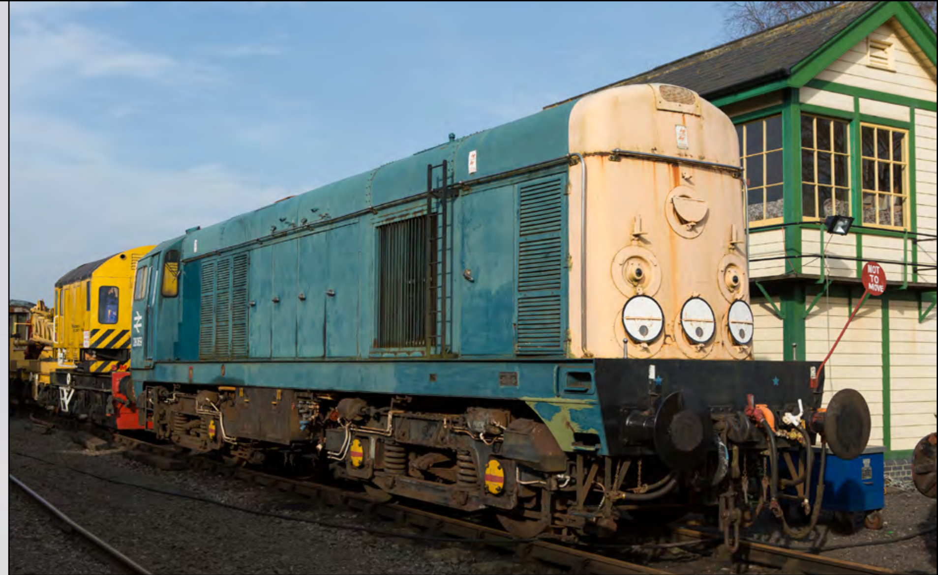
Right: Class 20 No. D8069 is seen next to the Mid Norfolks 10t 4w self-propelled diesel crane, built by Thomas Smith & Sons (Rodley) Ltd, No. DR81330. Jon Jebb
