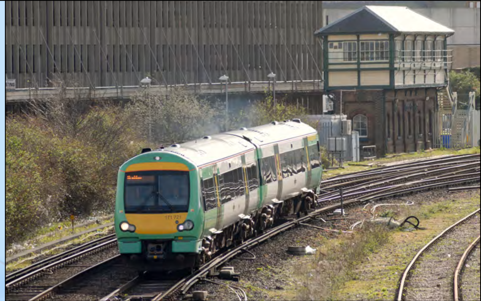
Above: The Saxby & Farmer-designed box at Eastbourne was one of several in England that was given Grade II listed status in 2013 and safeguarded. On March 22nd, Southern Railway's Class 171 721 leaves Eastbourne working the IG34 Ashford International - Brighton service after reversing at the terminus. The signal box was built in 1882 and became a power signal box in 1991 when the semaphore signalling was replaced by colour-light signals. Gary S. Smith
