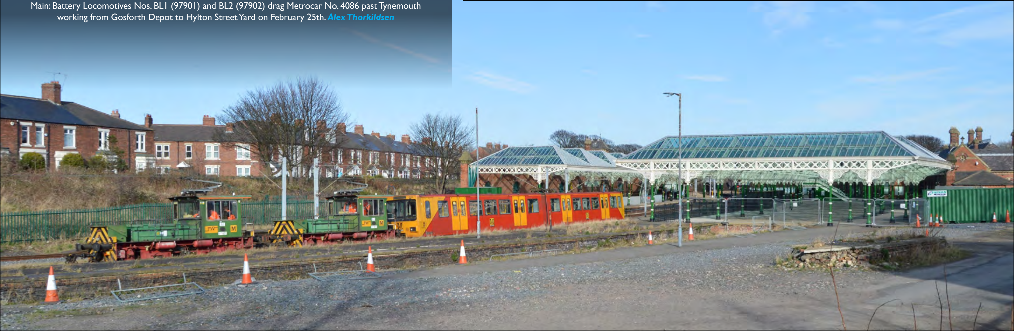
Right: Equipped with new pantographs for their upcoming mainline registry exam, Battery Locomotives Nos. BL1 (97901) and BL2 (97902) stand in Road 2 of Stoddart Street Sidings top'n'tailing refurbished Metrocar No. 4068, heading to Gosforth Depot after taking a detour here to charge for 45 minutes. Alex Thorkildsen
