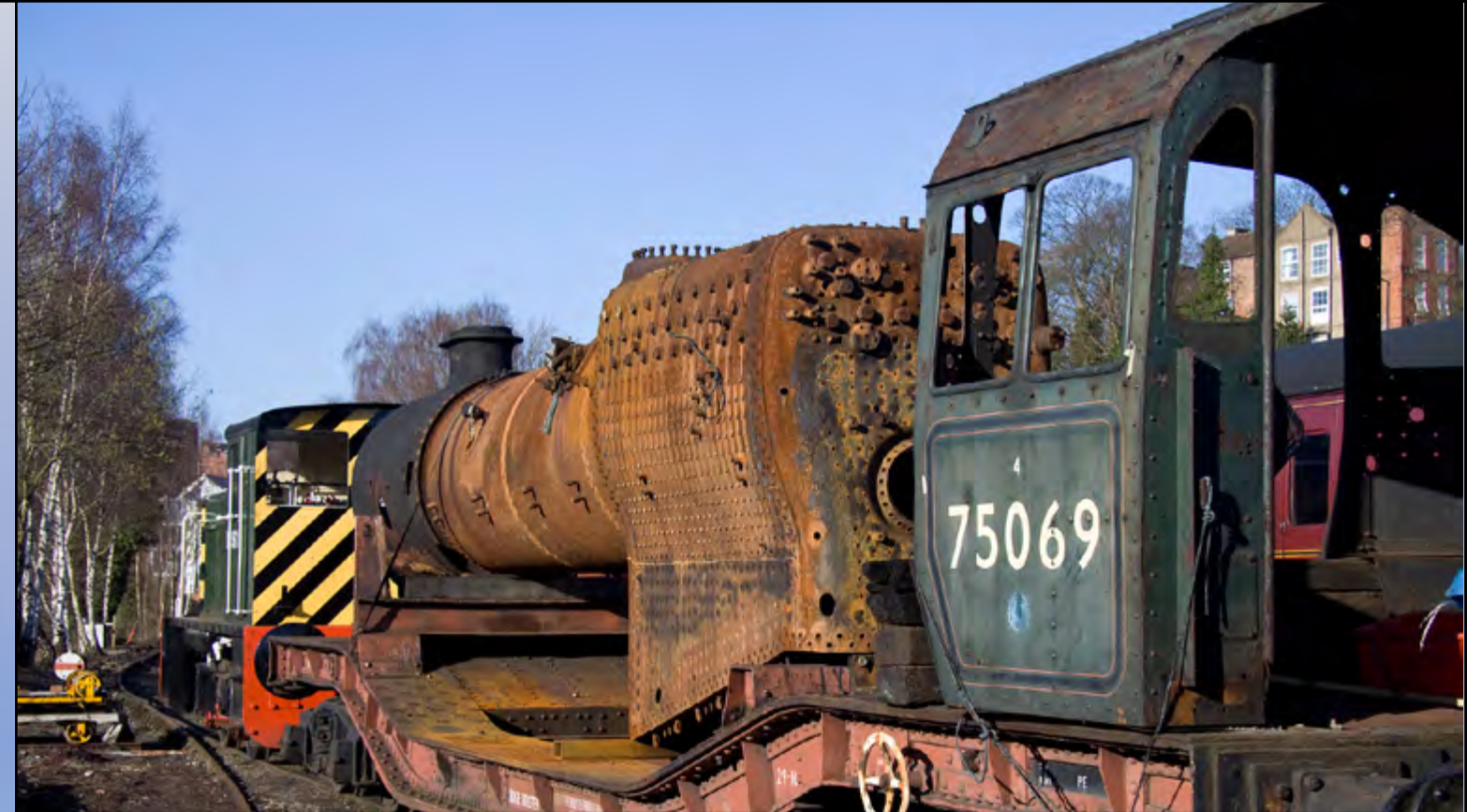
Above: Restoration work is continuing on BR standard Class 4 4-6-0 No. 75069 at Bridgnorth, seen here just cab and boiler whilst the frames are being worked on. Richard Hargreaves
