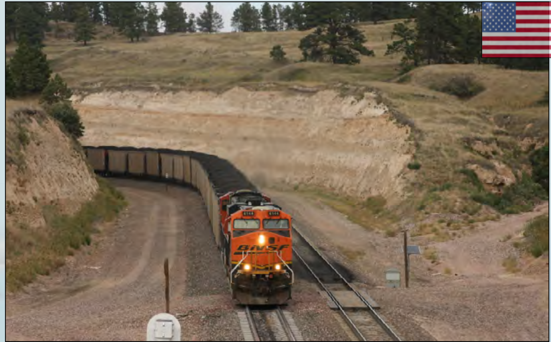
Right: At Crawford Hill, Nebraska, a BNSF coal loads struggles over the summit at Belmont. These 13,000 ton coal trains have to stop at Crawford to attach banking engines for the 15 mile climb up Crawford Hill. By the summit they are down to walking pace. Andy Pratt
