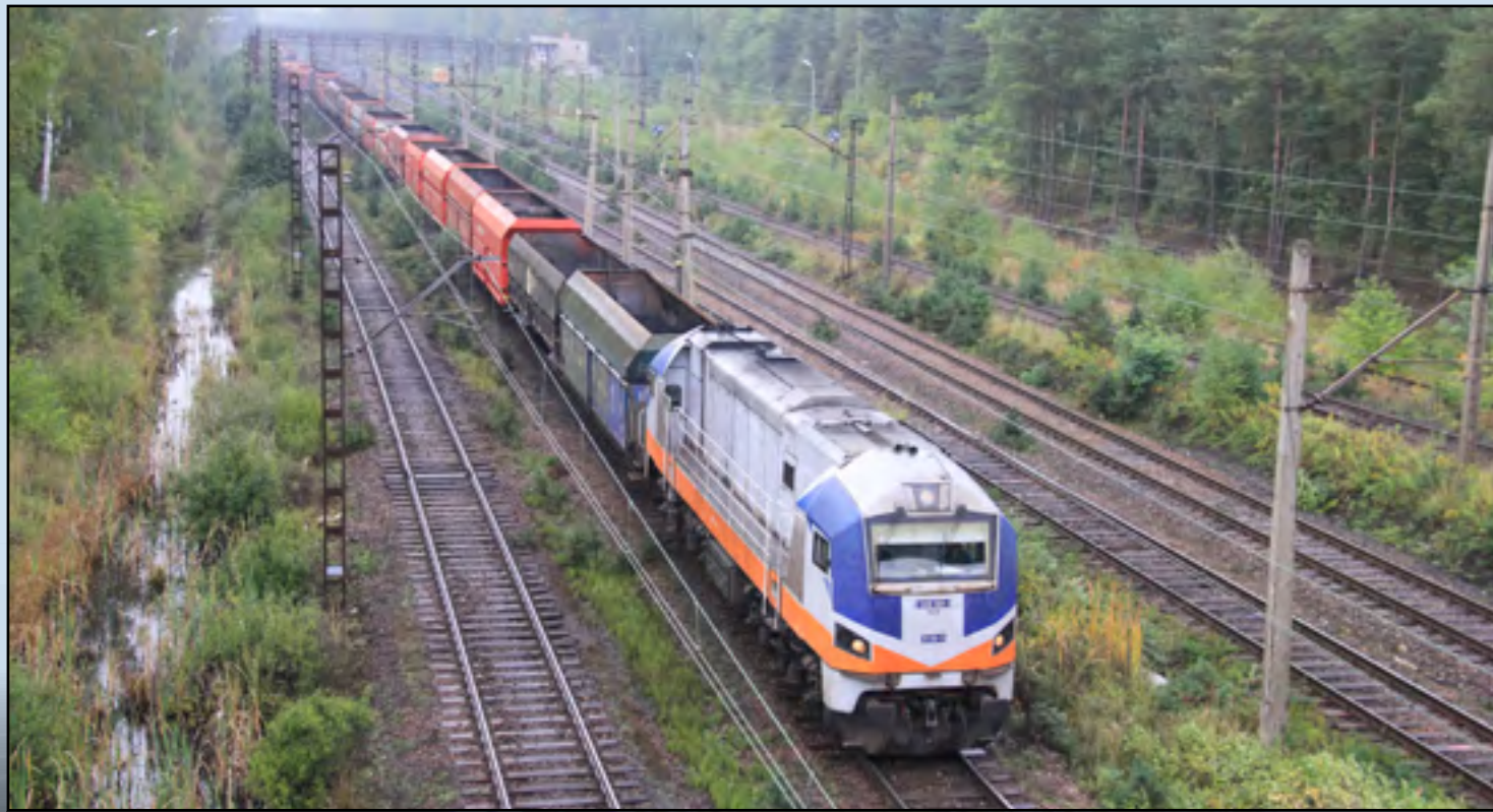
Above: DB Schenker Poland Class 311-D11 (92 51 3 640 021-3) works through Katowice Sosnowiec on September 26th. Amazingly these are rebuilds of the popular ST44 locomotives. Anton Kendall
