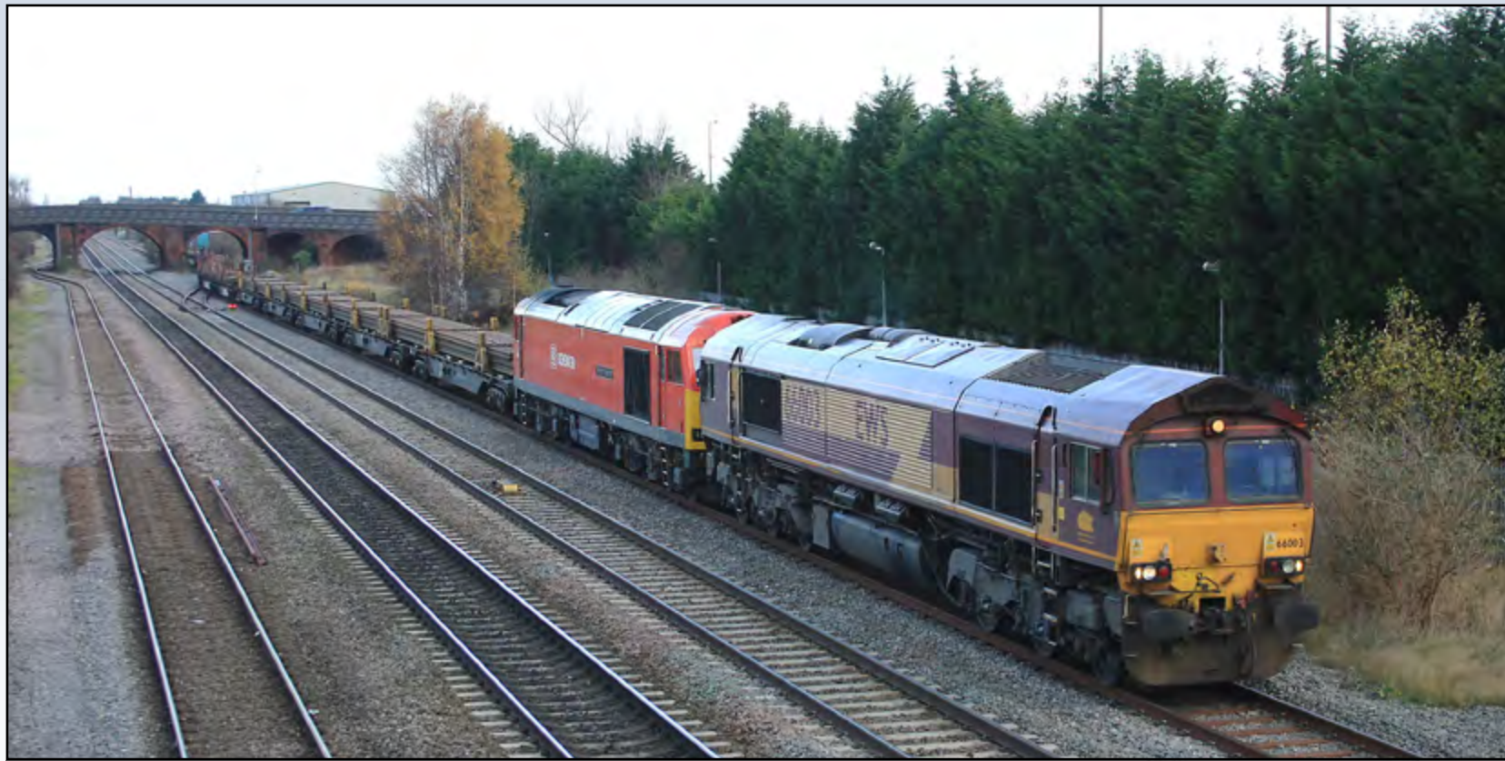
Above: On a dull December 6th, Class 66 003 and 60 059 are seen at the head of 6X01 Scunthorpe to Eastleigh with continuous welded rails, passing through Burton on Trent. Stuart Hillis
