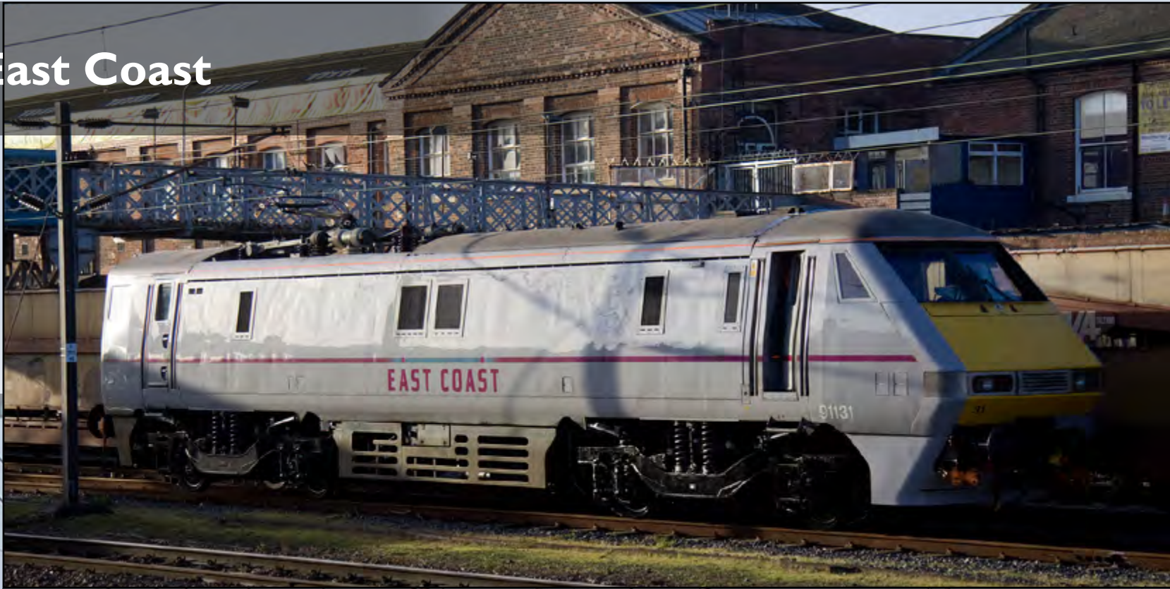
Above: On December 21st, Class 91 131 emerges from Wabtec Doncaster works having had attention to its bogies and wheelsets. Richard Hargreaves
