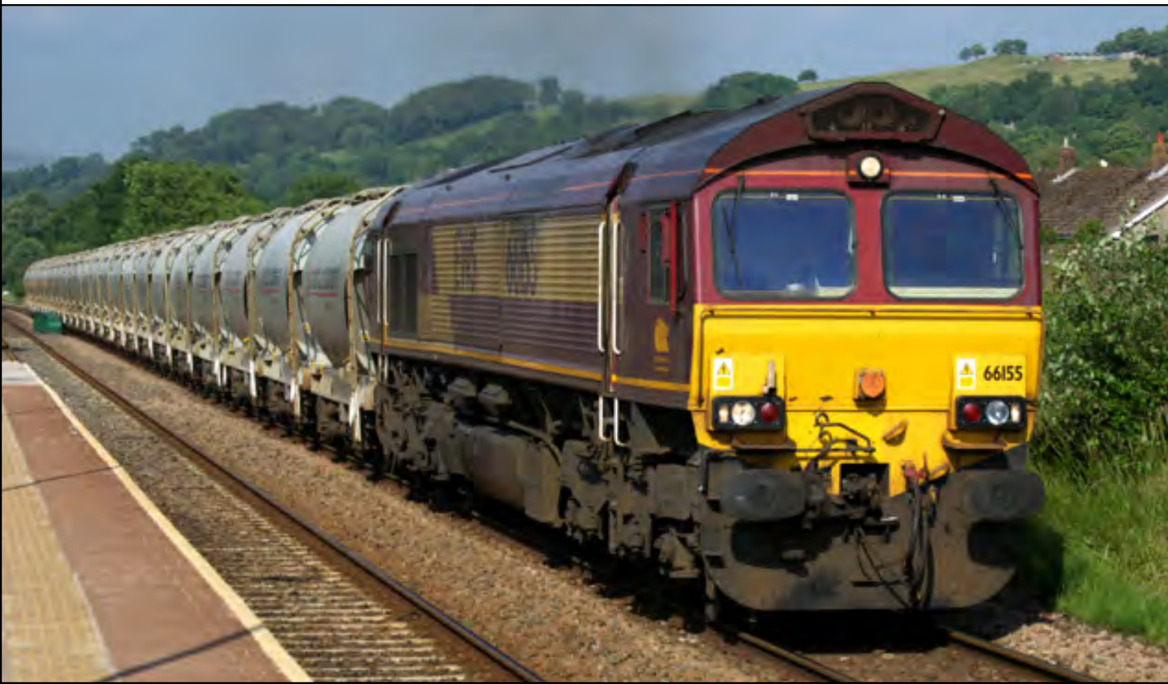
Below: Class 66 155 is seen climbing up the 1 in 82 Langho Bank hauling on the inaugural run of 6Z35 Clitheroe Castle Cement to Avonmouth with 1,200 tonnes of loaded cement on July 9th. Dave Felton
