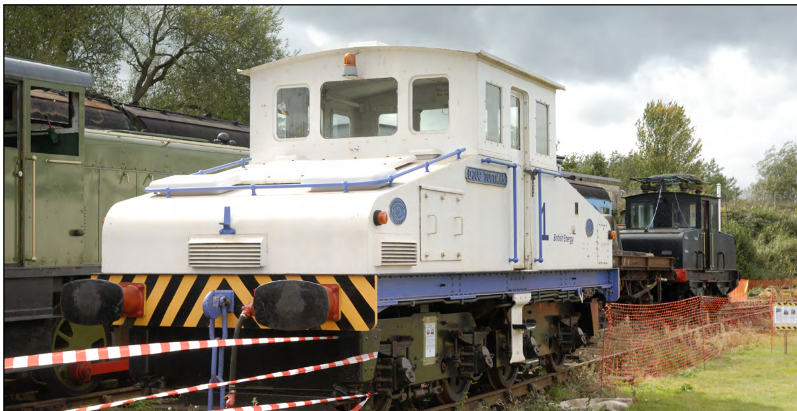
Below: Heysham electric locomotive No. 1 was originally Kearsley number 4, having been built by Robert Stevenson & Hawthorn in 1945 for the Lancashire Electric Power Company. After the Kearsley power station was closed in 1982, the locomotive was converted to battery power and moved to Heysham where it was named "Doug Tottman". It was the last working standard-gauge industrial electric locomotive in the UK, being retired by British Energy in 2009 and replaced by diesel traction. Gary S. Smith
