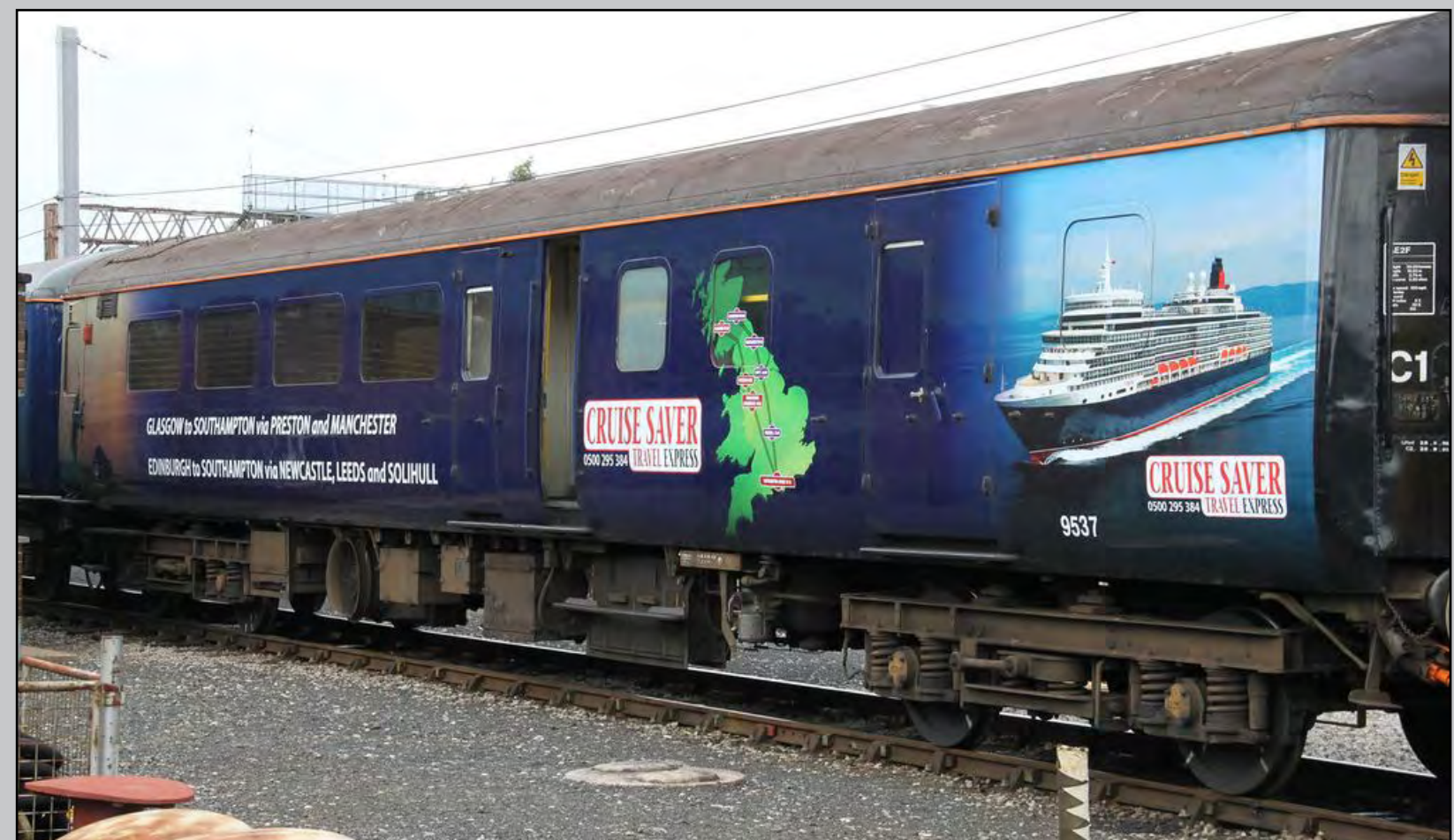
Below: BSO to baggage van. MK2f BSO No. 9537 has been converted to a baggage car for use on this service, with the removal of its seats to provide a large area for luggage/suitcases. 9537 has been in Virgin livery before being replaced by vinyls for the Cruise Saver Express. Robert Duff
