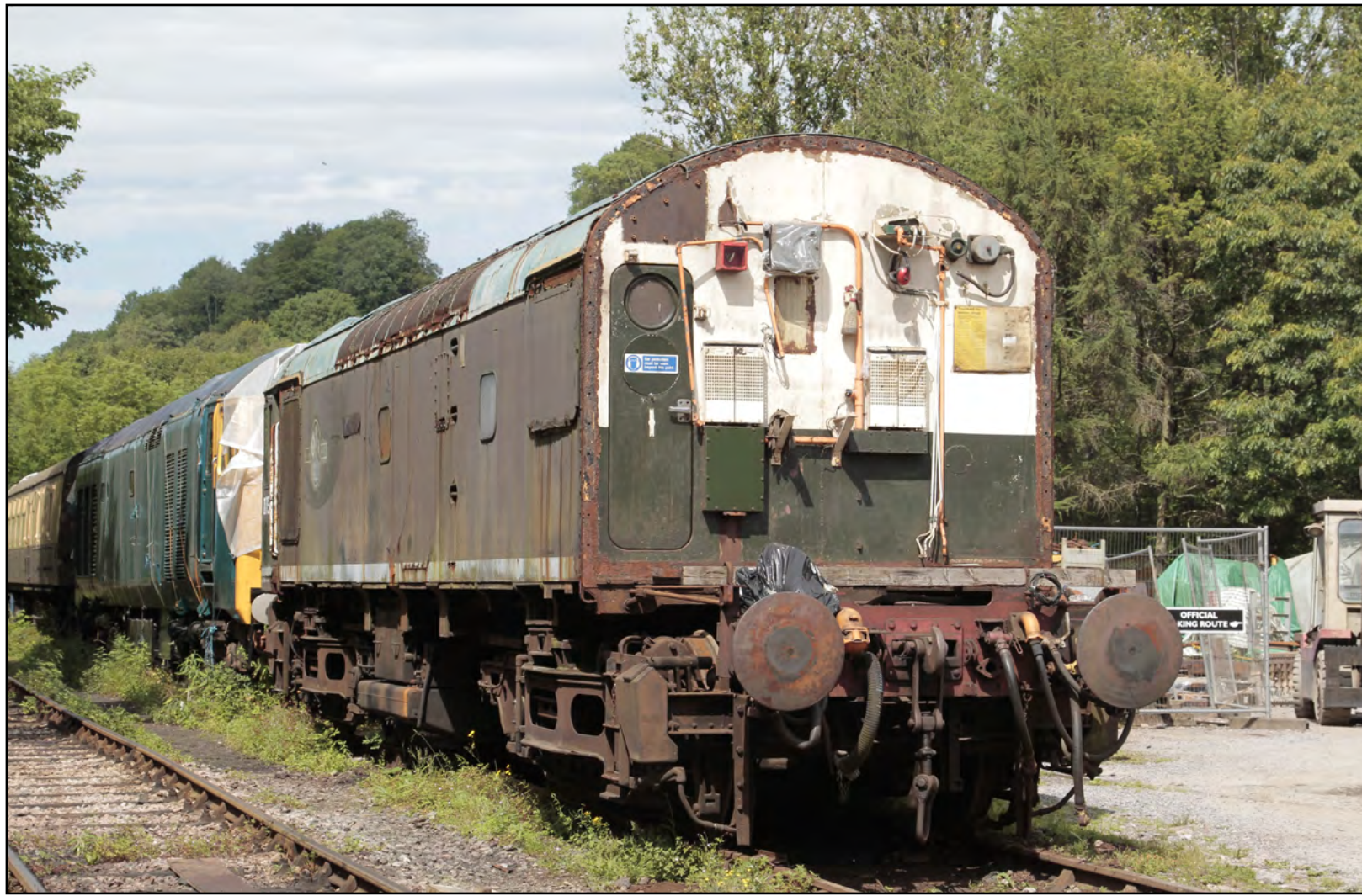
Above: Rat without a Cab - Class 25 No. D7541 is seen at Buckfastleigh in July after its cab was removed for much needed repairs. Andy Below: BR Class 122 DMU No. W55000 arrives into Totnes on July 26th. Class47
