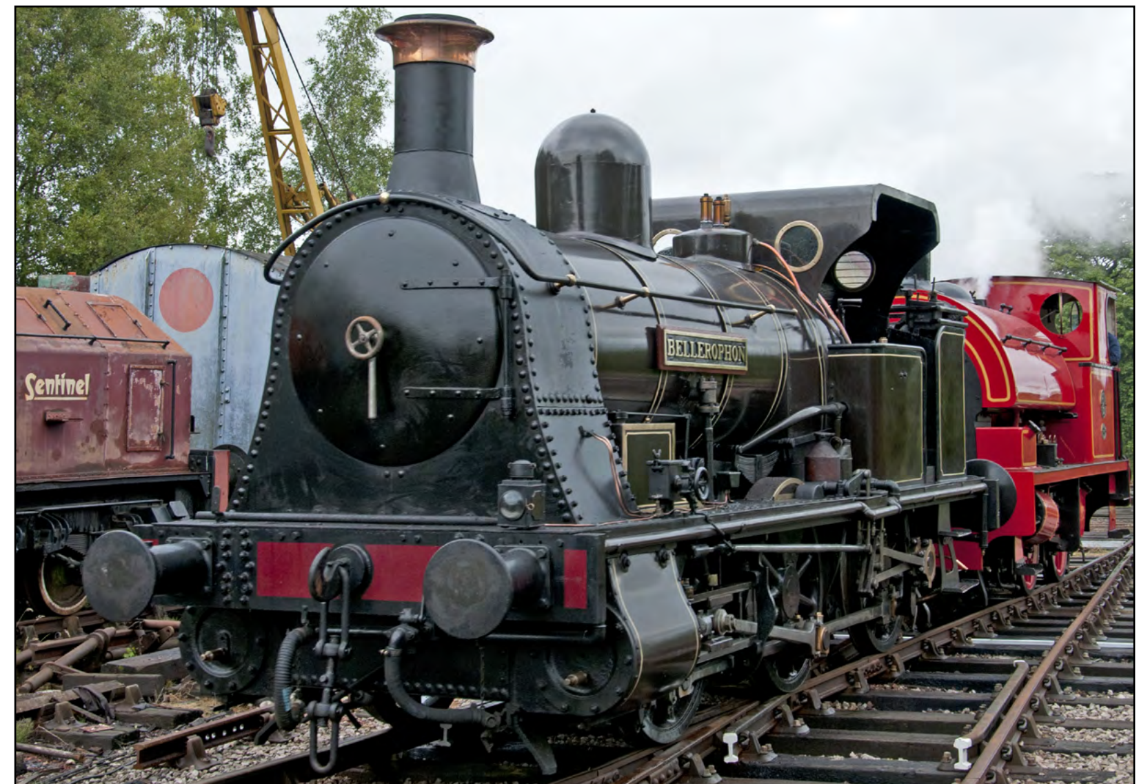
Above: Devonport Dockyard 0-4-0ST No. 19 is seen shunting at Foxfield Colliery. Richard Hargreaves Below: Haydock Foundry 0-6-0 well tank built in 1874, No. C "Bellerophon" rests at Caverswall Road. Class47
