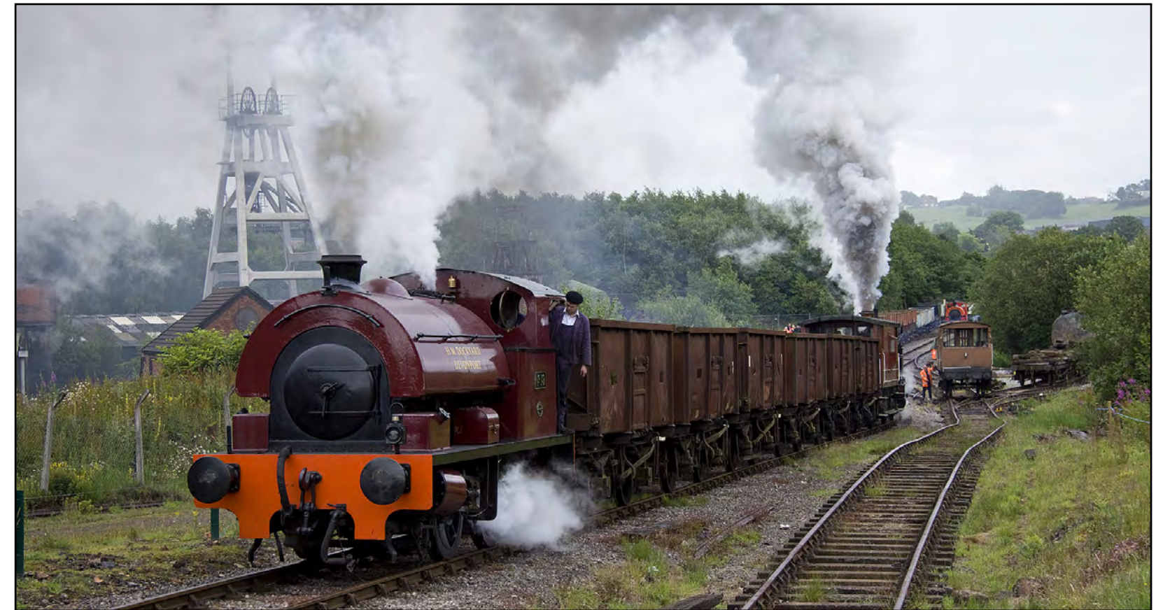
Above: Devonport Dockyard 0-4-0ST No. 19 is seen shunting at Foxfield Colliery. Richard Hargreaves Below: Haydock Foundry 0-6-0 well tank built in 1874, No. C "Bellerophon" rests at Caverswall Road. Class47
