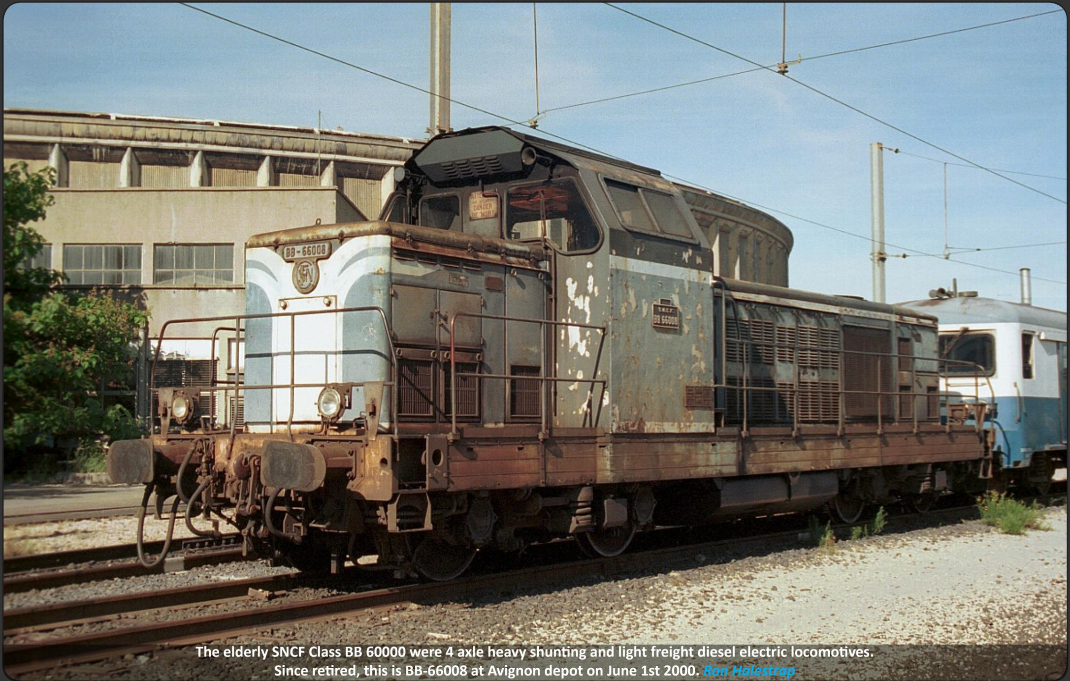
The elderly SNCF Class BB 60000 were 4 axle heavy shunting and light freight diesel electric locomotives. Since retired, this is BB-66008 at Avignon depot on June 1st 2000. [Ron Holestrap](#)
