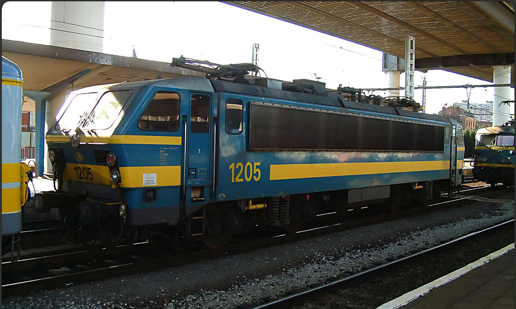
Belgium's SNCB Class 12 locomotives are dual-voltage (25 kV AC and 3000 V DC) and designed on the single-voltage Class 21. They were built to work freight and passenger services between Belgium and Lille in France. SNCB 1205 is seen at Charleroi on October 28th 2002. [Brian Battersby](#)
