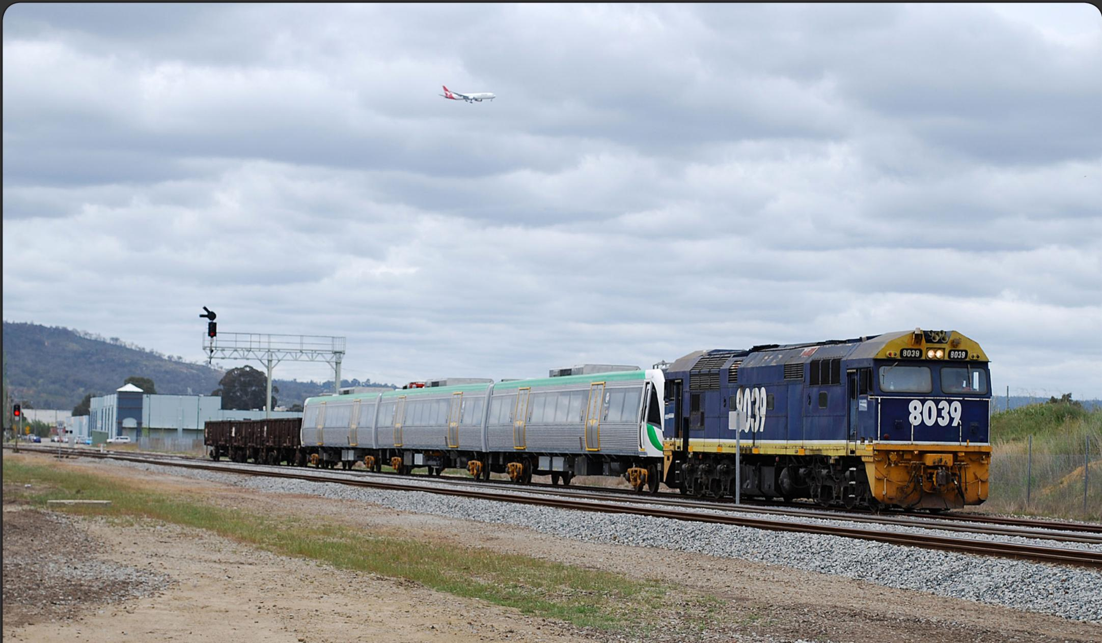
Class 80 Co-Co No 8039 shunts a newly arrived 'B' set EMU at Midland on October 19th. Still on the standard gauge transporter bogies that it travelled on from the manufacturer in Queensland. In the open wagons are the narrow gauge motor bogies that will be fitted prior to delivery to the suburban network in Perth.. [Colin Gildersleve](#)
