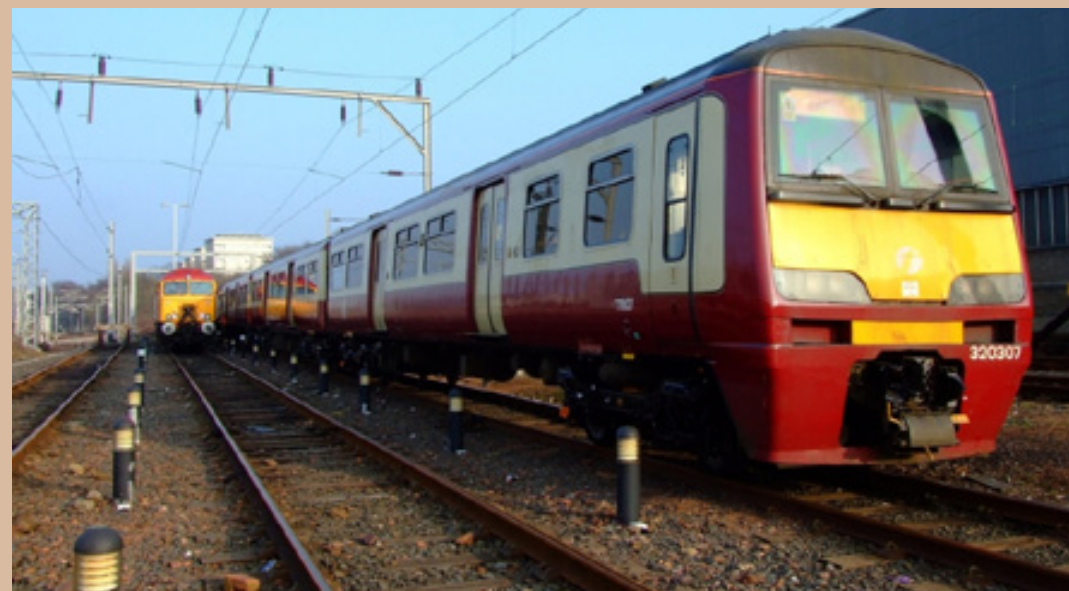
Class 320 307 is seen sitting outside in the yard at Shields T.M.D. having just come out from Glasgow Works, Springburn after going through a C4 overhaul. The unit had just been brought back from Glasgow Works some 3 hours later than planned running as 5D02 by Class 57 307 which is seen sitting next to the unit.
