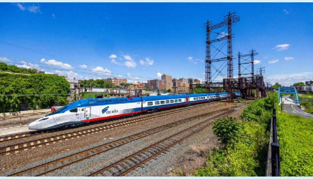
parts for preventative and corrective maintenance, component overhauls, training, maintenance and support to maximize fleet availability. Equipped for condition-based and predictive maintenance, Alstom has embedded each train set with nearly 100 sensors to monitor wear and tear and predict when critical parts need to be serviced or replaced. Alstom has also guaranteed that it will supply any spare part within eight hours of when it is needed.
