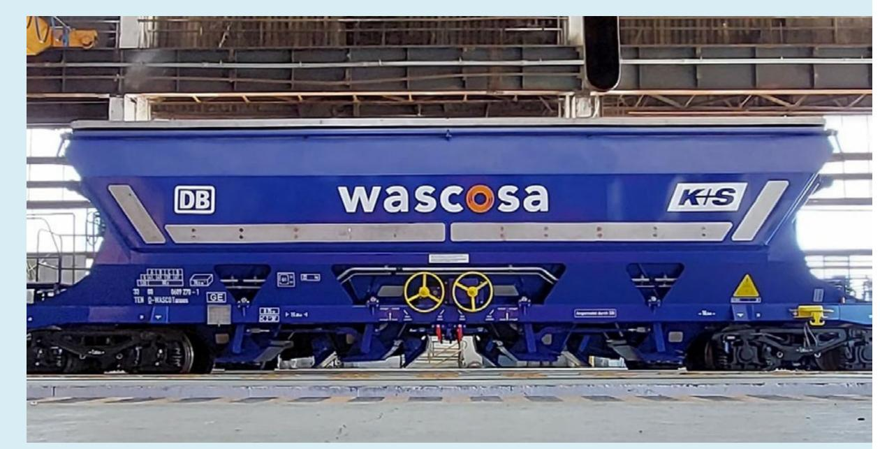
The stainless steel protects the paint, which would otherwise flake off. Corrosion caused by the load is avoided and the durability of the wagon is significantly increased.
