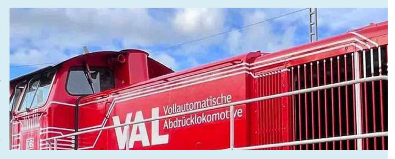
GmbH, both wholly owned subsidiaries of Robert Bosch GmbH, for the series development of the fully automatic push-pull locomotive. Bosch Engineering is developing an automation unit for fully automatic push-pull operation, including sensors and algorithms for environmental detection. ITK is responsible for developing the operator workstation on the infrastructure side, which implements the input and management of
