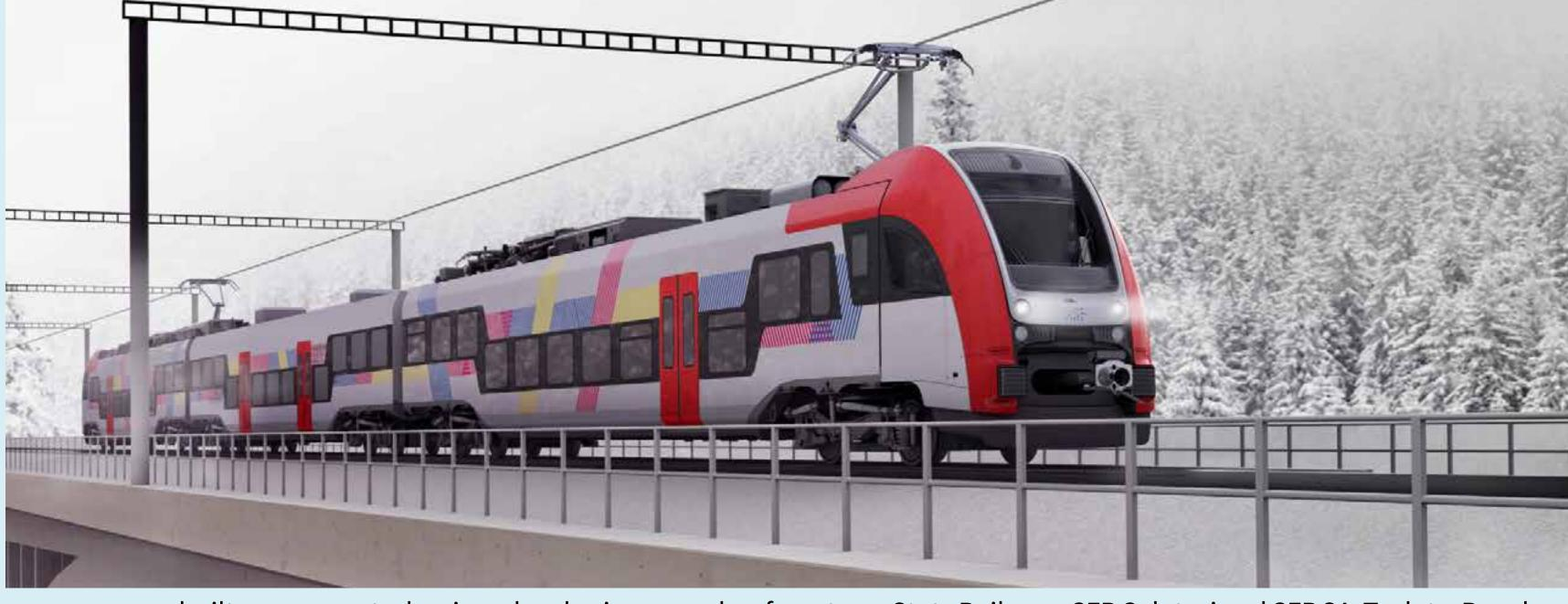
built on separate bogies, developing speeds of up to 160 km/h, with 192 seats in 1st and 2nd class, allowing barrier-free operation of 550 mm platforms, powered by AC 25kV catenary and equipped with the Romanian PZB 90 safety system.
