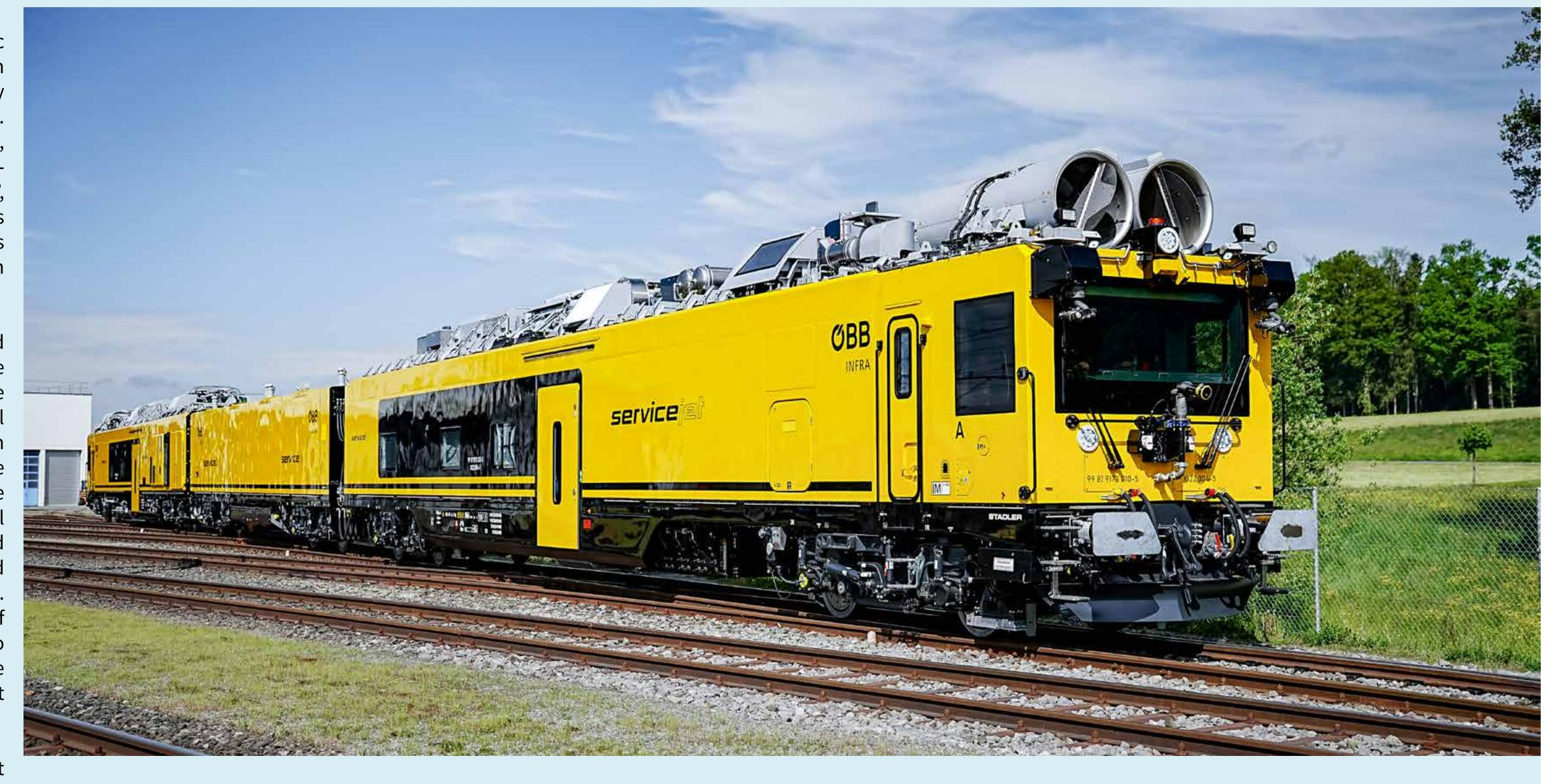
access along the entire train. 18 seats are fitted with SCBA brackets for firefighters. An HVAC system with special filters protects people on the train from smoke gases. What is more, the entire train is pressurised, which means that there is a slight overpressure inside to keep it free of smoke in tunnels. The front part of the train where the driver's cab is located is protected by a water spray system on the outside.
