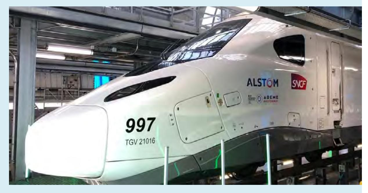
The future INOUI TGV promises to usher in a new era in TGV maintenance. It will be a communicating trainset that will provide permanent remote access to technical data and clear information on the state of each of its components. This will make it possible to plan maintenance operations based on the actual condition of the components, and to anticipate breakdowns in doors, air conditioning and, more generally, all the systems that contribute to train operation and passenger comfort.
