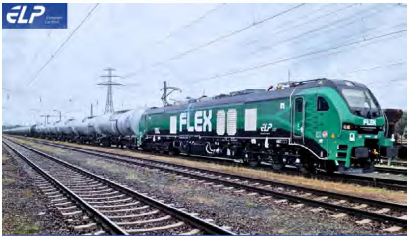
customer," European Loc Pool ordered the first ten Euro9000 locomotives from Stadler in May 2019. The first version with 1.9 MW of diesel and 9 MW of electric power at 500 kN tractive effort will be used in Germany, Austria, the Netherlands, Italy, Belgium, and Switzerland. Subsequently, the locomotive's area of operation will be expanded to other countries and corridors.
