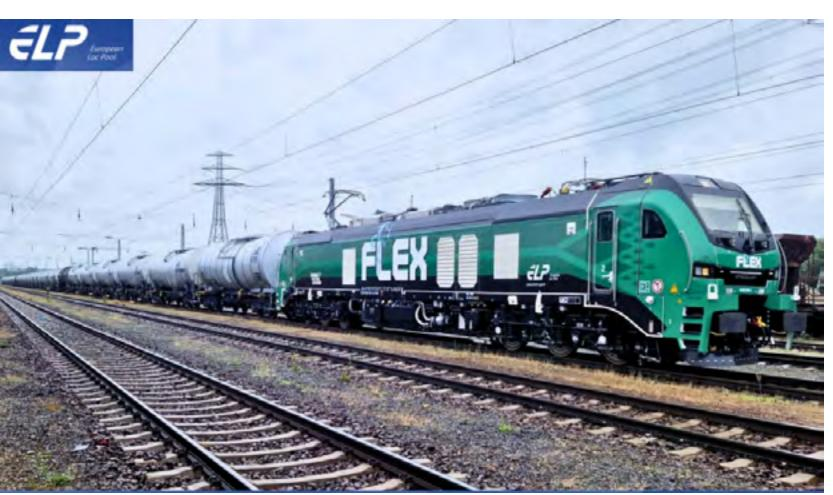
customer," European Loc Pool ordered the first ten Euro9000 locomotives from Stadler in May 2019. The first version with 1.9 MW of diesel and 9 MW of electric power at 500 kN tractive effort will be used in Germany, Austria, the Netherlands, Italy, Belgium, and Switzerland. Subsequently, the locomotive's area of operation will be expanded to other countries and corridors.
