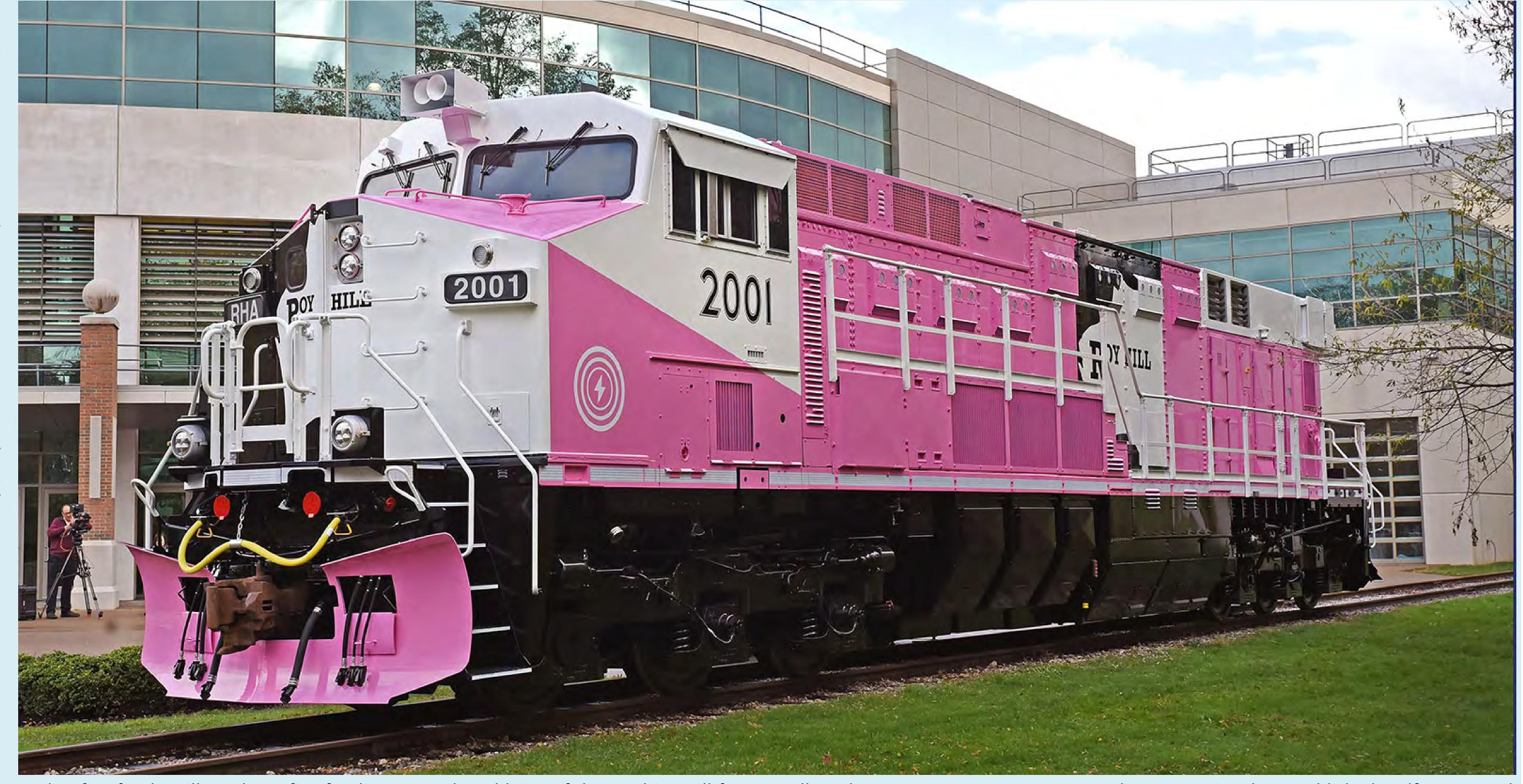
only a first for the Pilbara, but a first for the mining industry. The technological smarts that have gone into the development of the loco makes it well suited for our rail network. By using regenerative braking, it will charge its battery on the 344 kilometre (214 mile) downhill run from our mine to port facility and use that stored energy to return to the mine, starting the cycle all over again. This will not only enable us to realise energy efficiencies but also lower operating costs."
