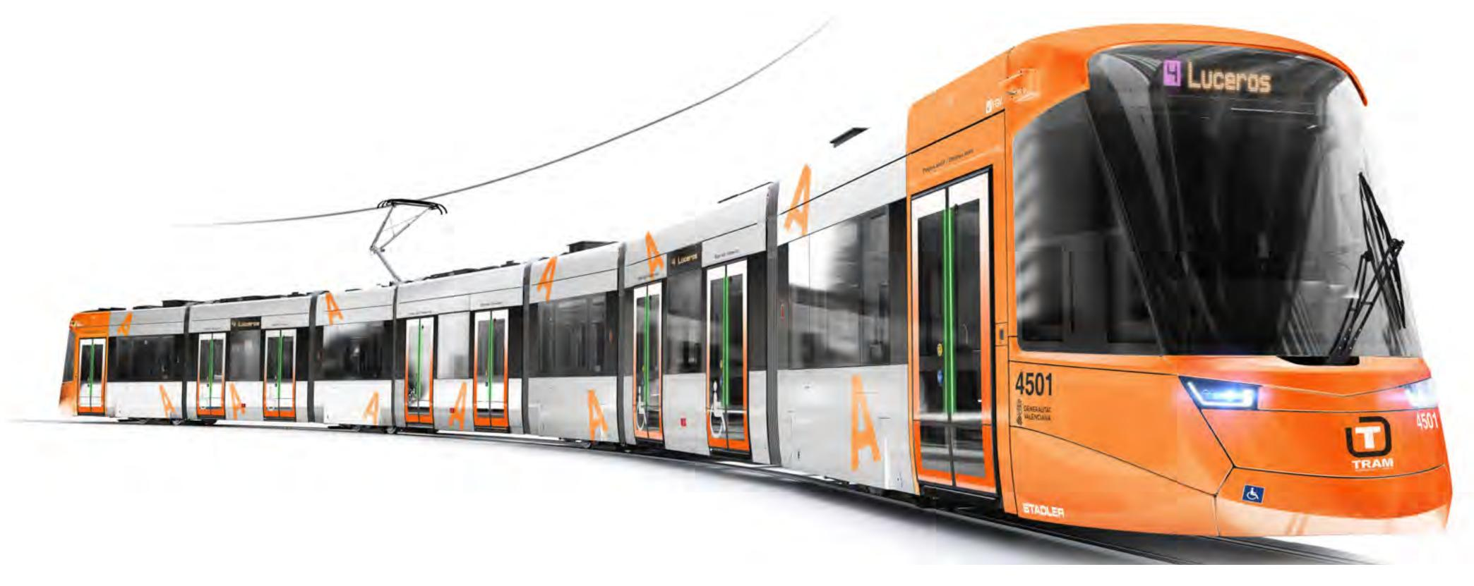
features include Innovative design regenerative braking with energy recovery, an efficient AC traction system with one inverter per axle providing a high level of redundancy and increased reliability, the HEP system to supply energy to the train, as well as the possibility to install either an UIC or an automatic coupler.
