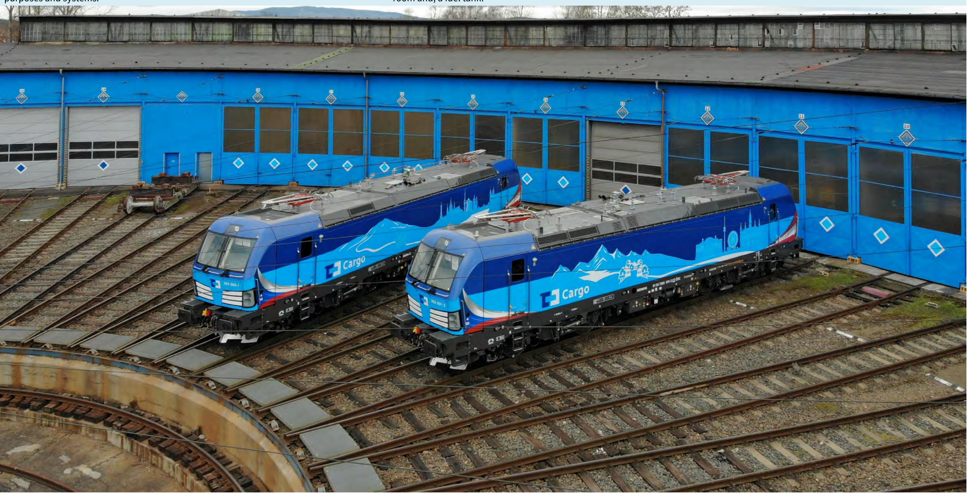
The new engines are equipped with an auxiliary diesel engine (DPM – Diesel Power Module) for operation on handling tracks and sidings without traction catenary line or when shunting. The DPM module consists of a 180-kW diesel unit located in the engine room and, a fuel tank.
