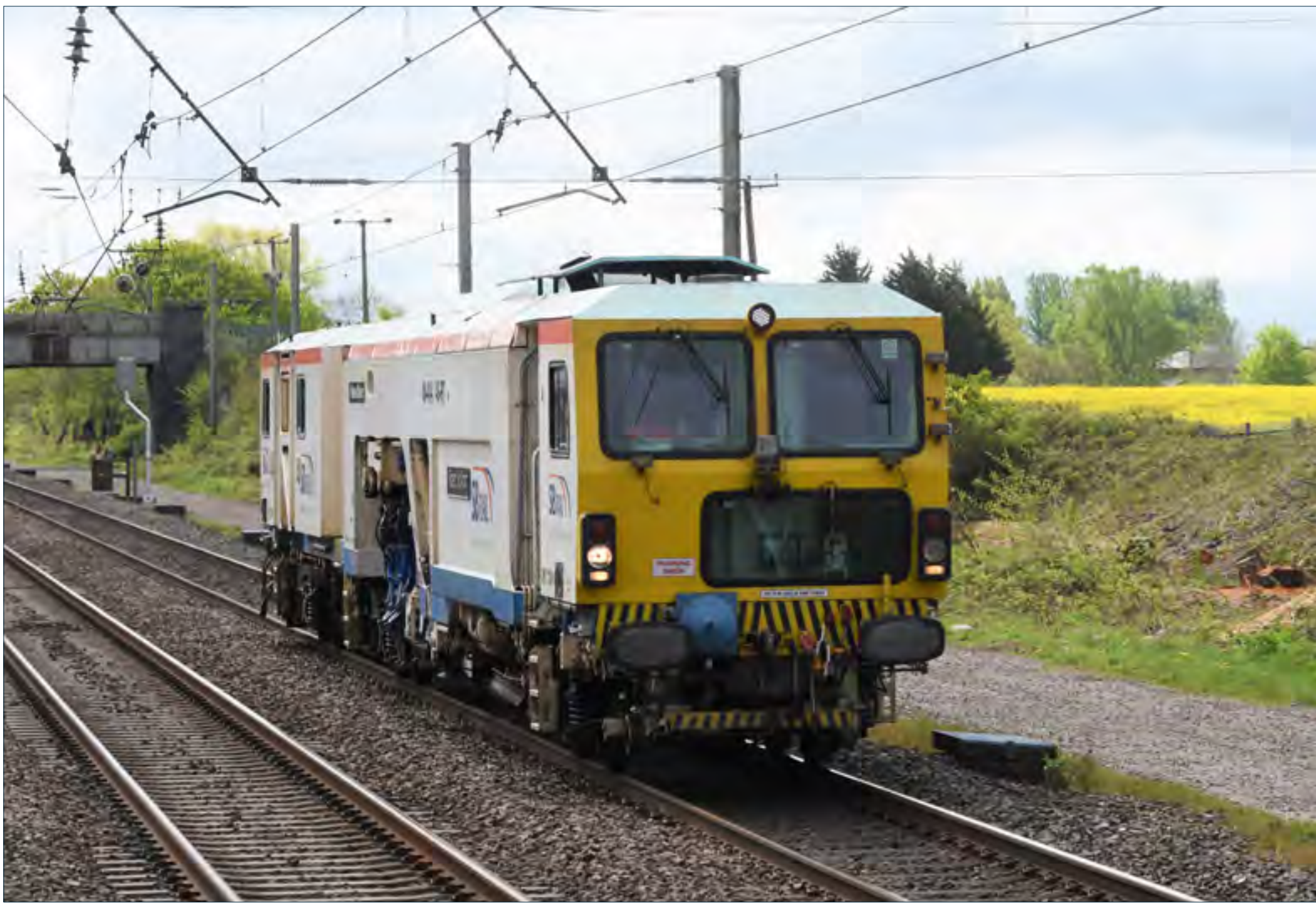
SB Rail’s Plasser & Theurer 08-4x4/4S-RT Switch & Crossing Tamper No. DR73914 speeds past Coppull. John Sloane
