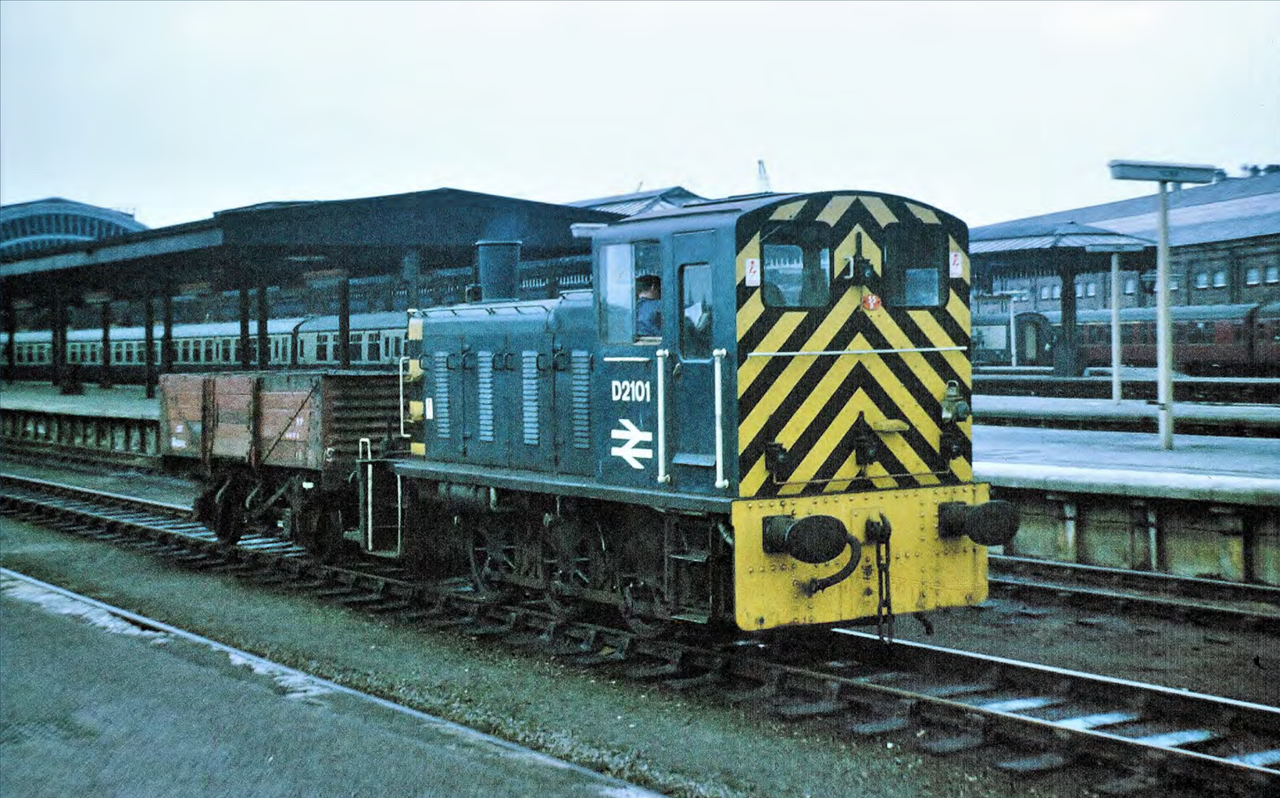
BR Class 03 No. D2101 with a match wagon acts as York station pilot on March 27th 1968.
