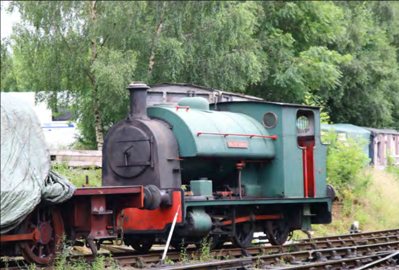
W. G. Bagnall 0-6-0ST No. 2221 'Lewisham' built in 1927, is pictured stored in the yard at Caverswall Road awaiting overhaul after its boiler ticket expired. Class47
