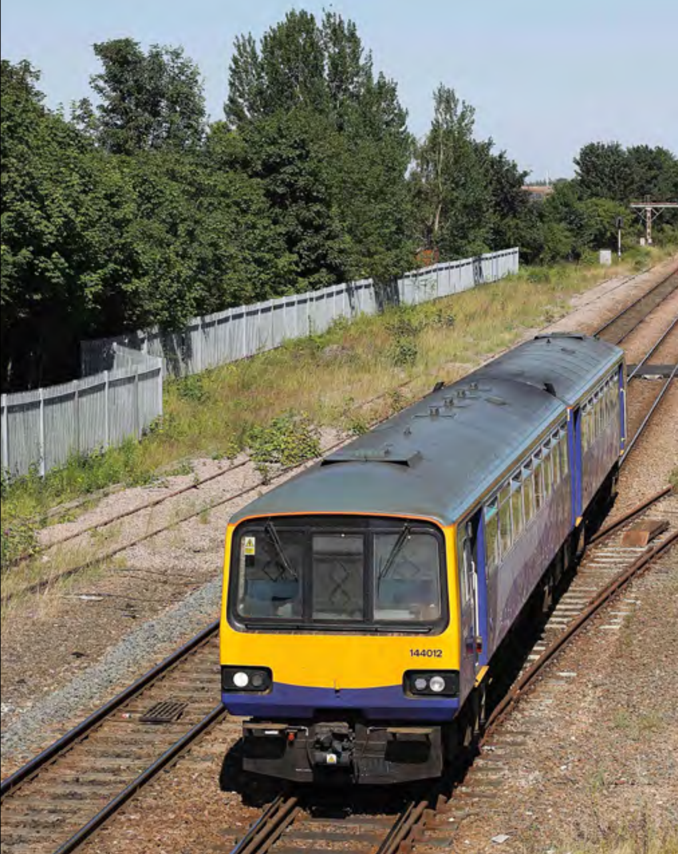
Refurbished Class 144 012 'Evolution' approaches Pontefract Monkhill with the 15:13 Knottingley - Leeds service on July 19th. It has new seating, lighting, toilets and is seen as a low cost option to new units - oh joy!. Nick Clemson
