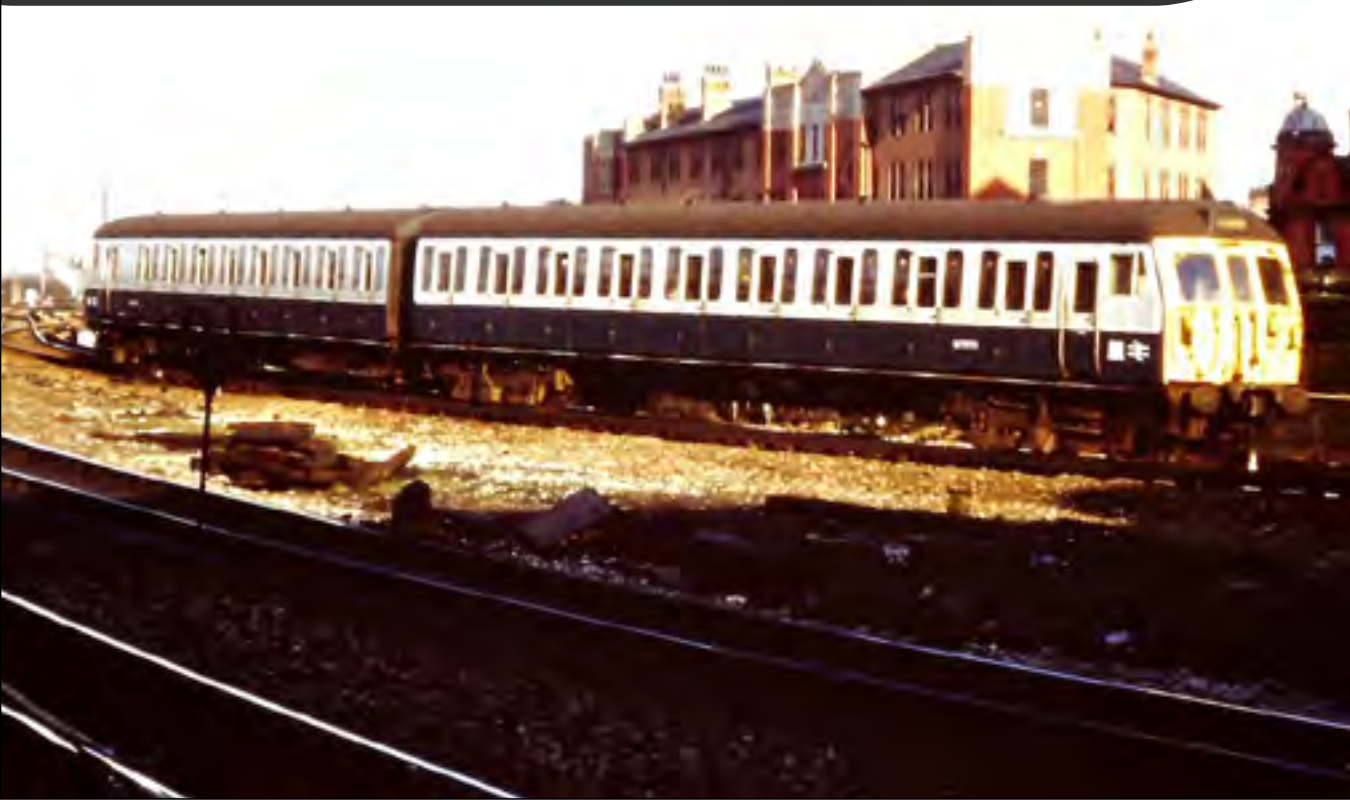
Before Metrolink: a Class 504 EMU is seen approaching Manchester Victoria station with a service from Bury in October 1982. These EMUs were introduced in 1959 and worked services until 1991, when the line was closed for conversion from heavy to light rail. Keith Chapman
