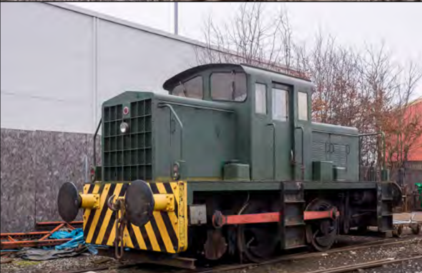
Vanguard 0-4-0 diesel hydraulic shunter. Built by Thomas Hill (Rotherham) Ltd. Brian Battersby
