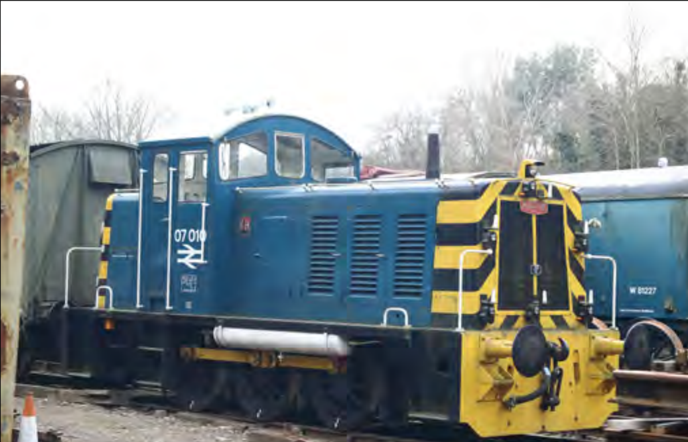
BR Class 07 0-6-0DE No. D2994 (07 010) awaiting repairs following electrical failure, is seen in the yard at Bitton. Class47
