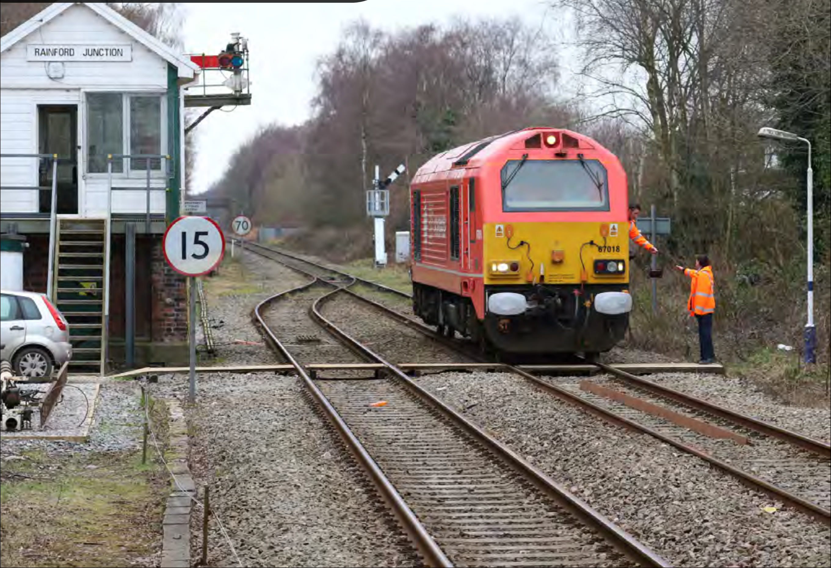
Class 67 018 is seen at Rainford Junction on March 22nd working 0Z70 Knowsley - Wakefield K Whitams Cobra route learner. The loco had just come off the single line and was handing the token back to the signalman. Alan Rigby
