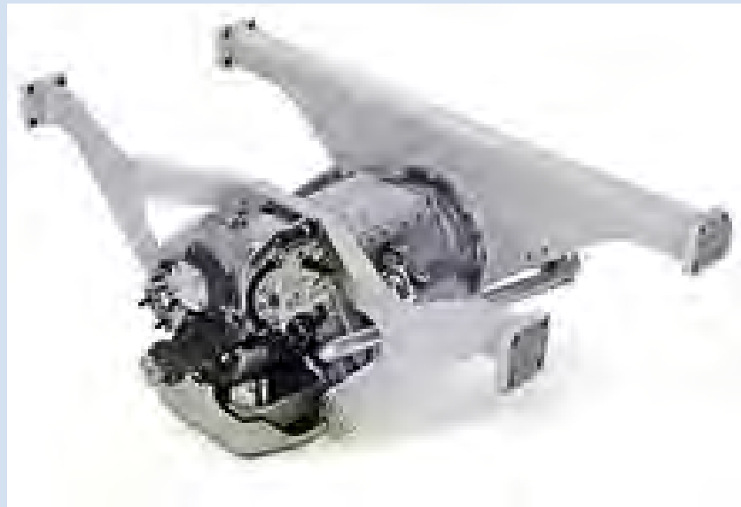
Photo: Voith DIWARail transmission with support frame for easy installation.
