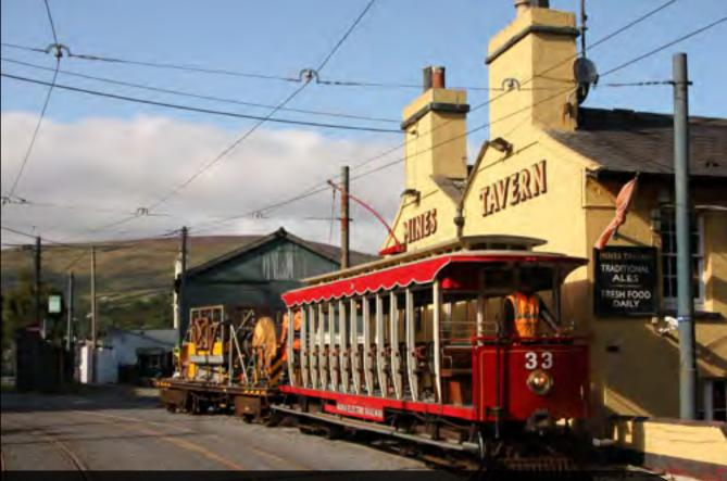
Manx Electric Railway car No. 33 works a permanent way electrification train past
