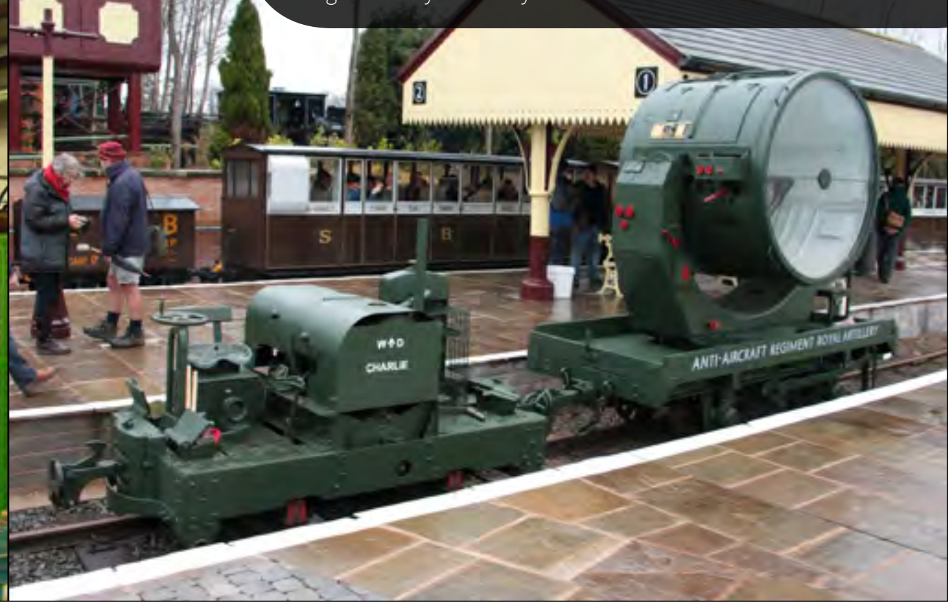
'CHARLIE', a diminutive 2 foot gauge petrol engine Simplex in War Dept. livery with mobile searchlight from the Anti Aircraft Regiment Royal Artillery. Stuart Hillis
