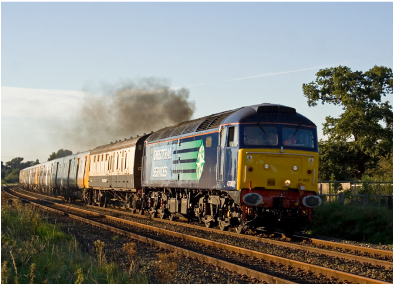
Above: 47802 passes Rowton on the 6th September with 7X47 Birkenhead North EMU Depot - Crewe CS unit move. Several 507/508s were being taken to various locations for tyre turning owing to excessive wheel wear. David Dawson
