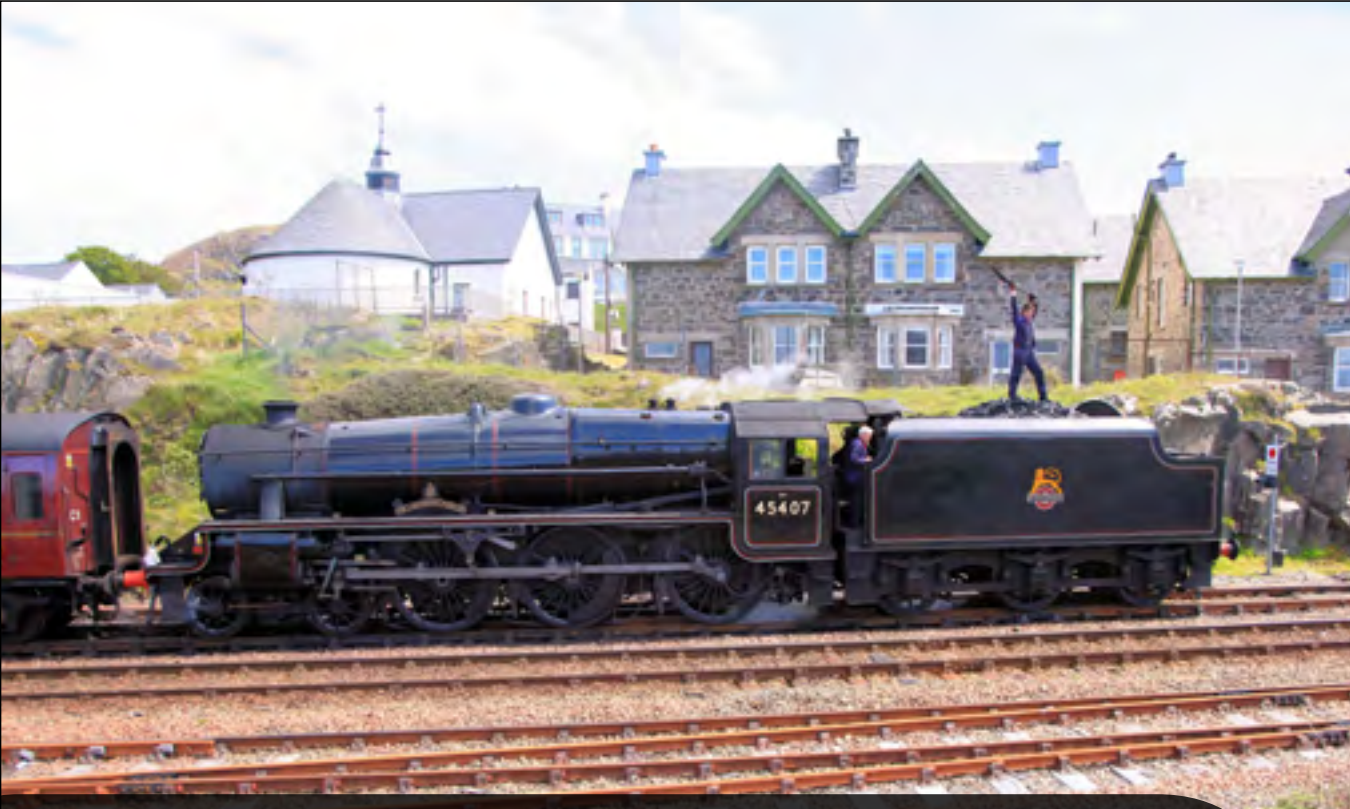
LMS Stanier Class 5 4-6-0 45407 'The Lancashire Fusilier' stands in Mallaig station on June 12th. The fireman is standing on the tender, shovel aloft, with the magnetic aerial attached in order that the driver can get a wireless link to speak to the signaller. Ah, the nostalgia of steam! Neil Pugh
